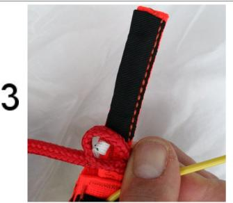
... thread the white loop through the loop on the end of the brake line...
