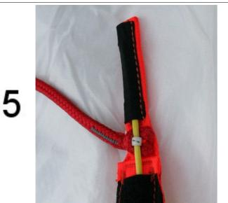
Insert the yellow cable inside the protective sleeve and pull on the brake line to place the system under tension.
