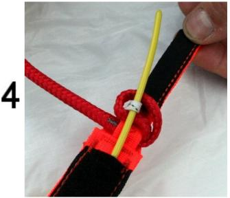
... and lock the system by passing the yellow cable through the white loop.
