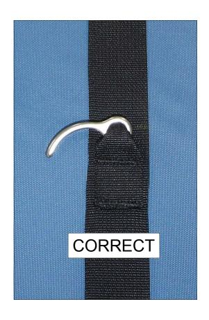
This would be considered a proper relationship between pin and pin retainer tab. With this relationship the pin would be allowed to rotate freely in the closing loop. The applied force (from pilot chute and bridle) would go directly to sliding the pin from the closing loop.
